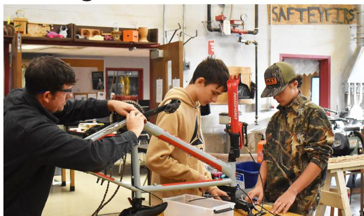
Earlier in the year, Mr. Tracy asked around for discarded bikes no longer in use so his engineering students could use them for a tech project. After doing some cutting, welding, grinding, and piecing together, the engineering class produced a bike-powered tennis ball launcher. Much like a pitching machine, the launcher worked better than anticipated and may end up being used to power other projects throughout the year. What a great way to turn trash into tech!
